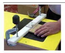
Once the fence has been clamped into position, use your wood sample and check to make sure that the pilot bearing on the bit has been isolated. In other words the bearing has to be even with the out-feed and the in-feed of the table fence.
