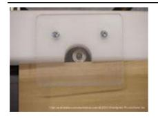
Move the in-feed side of the fence into position. Using a straight piece of material position the bearing flush with the out-feed and in-feed of the table fence. See photo.
