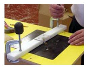
Hold the fence in this position and clamp the in-feed side. See photo.
